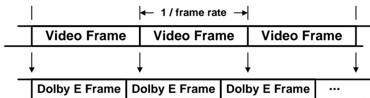
**Figure 5-2** Unsynchronized Dolby E Frames
