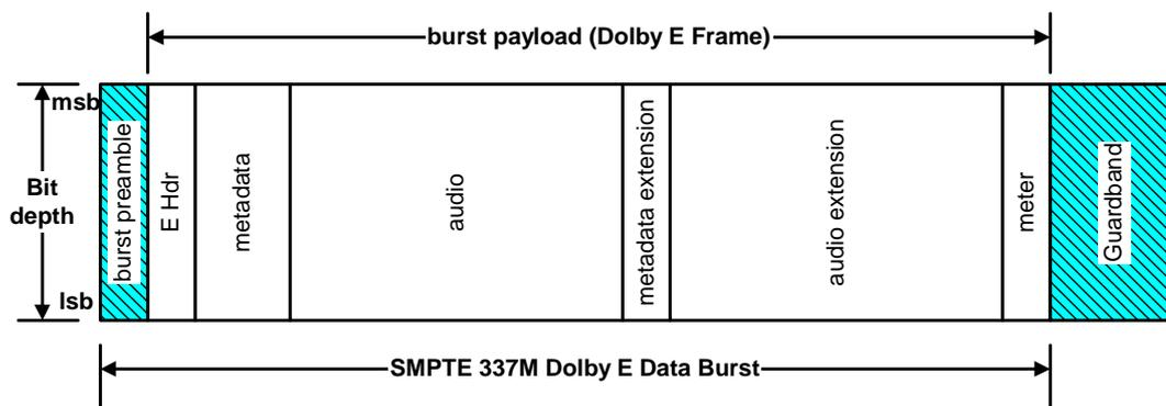
**Figure 4-4** Dolby E Frame with SMPTE 337M Transport Header
