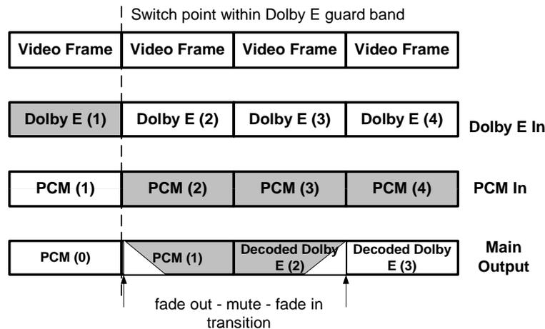
**Figure 5-9** Dolby E to PCM Transition
