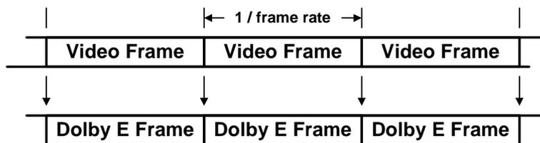
**Figure 5-1** Synchronized Dolby E Frames
