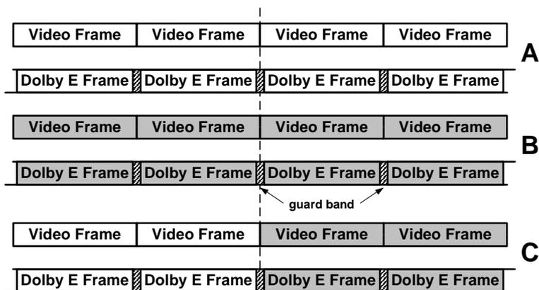
**Figure 5-5** Glitchless Switch/Edit of Phase-Aligned Dolby E Bitstreams
