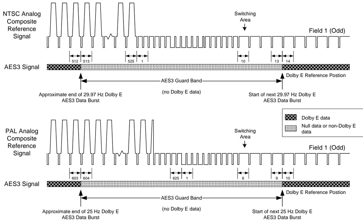
**Figure 4-8** AES3 Dolby E Data Burst Location with 5% Guard Band
