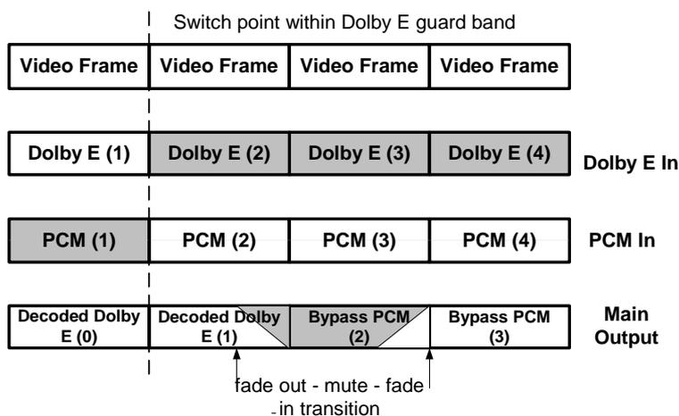
**Figure 5-8** PCM to Dolby E Switch
