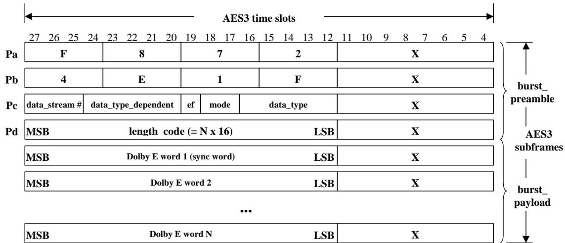
**Figure 4-6** Mapping Dolby E to AES3 time slots (16-bit mode)
