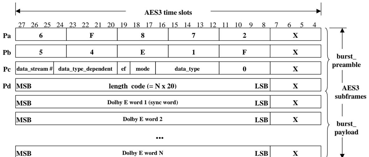
**Figure 4-7** Mapping Dolby E to AES3 time slots (20-bit mode)
