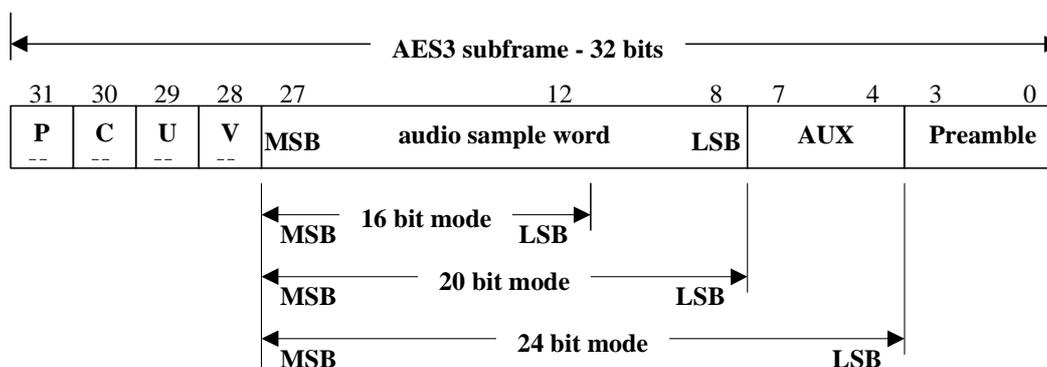
**Figure 4-5** Mapping Data Burst Segments to AES3 Subframes
