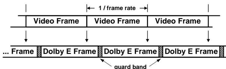
Figure 5-4 Non-Phase-Aligned Dolby E Frames
