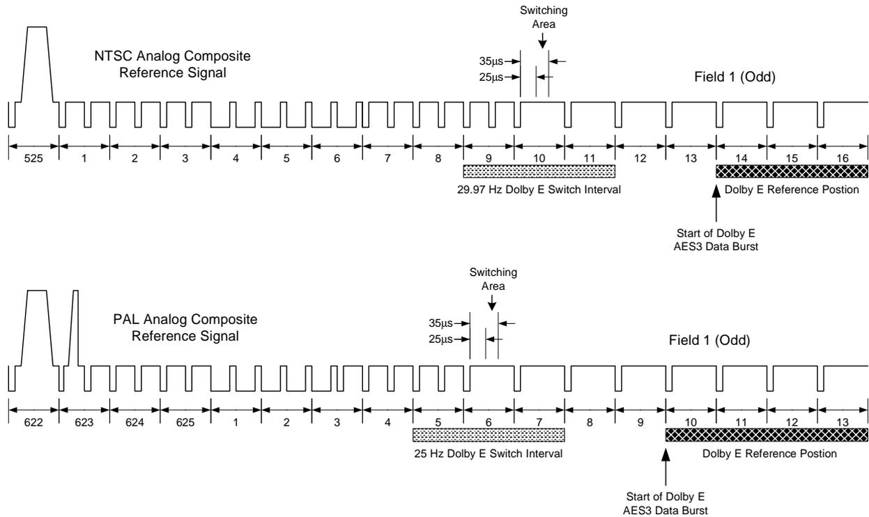
**Figure 9-2** AES3 Routing Switcher Dolby E Switch Interval
