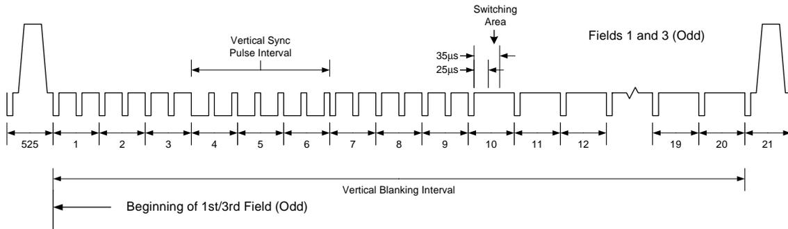
**Figure 4-1** NTSC Composite Vertical Blanking Interval
