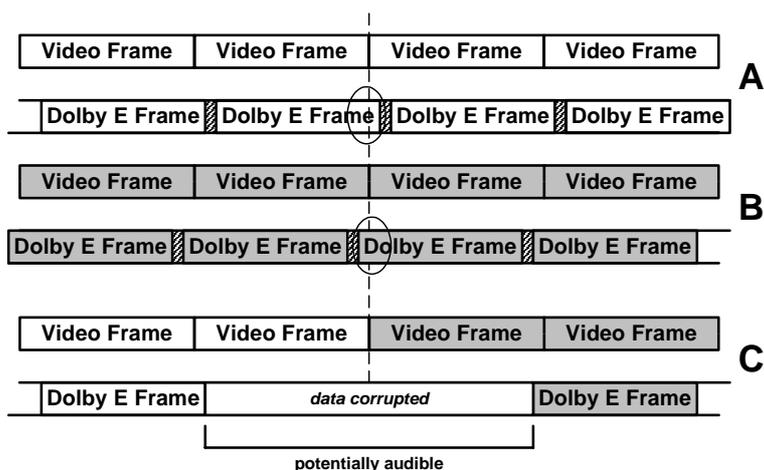
Figure 5-7 Switch/Edit of Non-Phase-Aligned Dolby E Bitstreams (Example 2)
