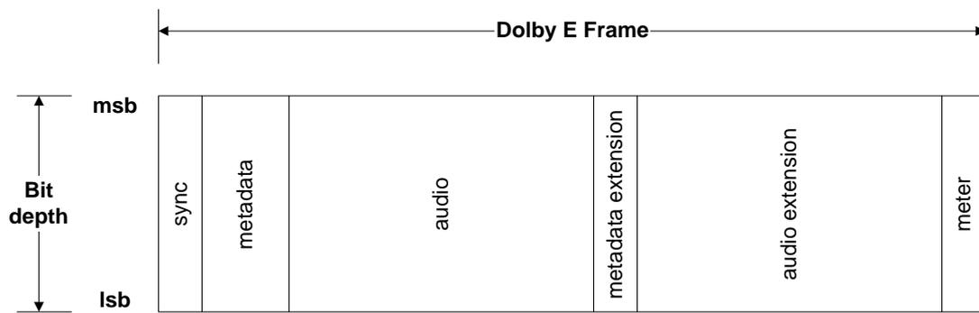
**Figure 3-4** Dolby E frame structure, low frame rate
