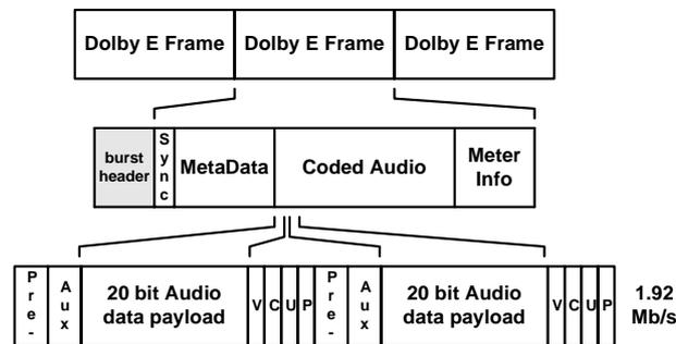
Figure 3-1 AES3/Dolby E Packet Structure
