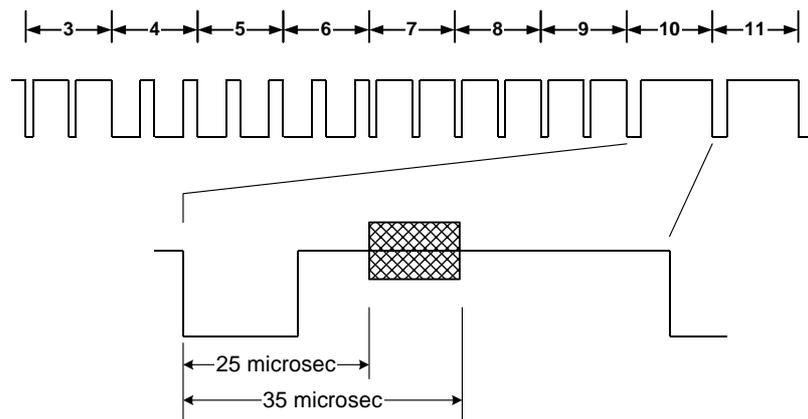
**Figure 4-3** NTSC Composite Vertical Interval Switching Area
