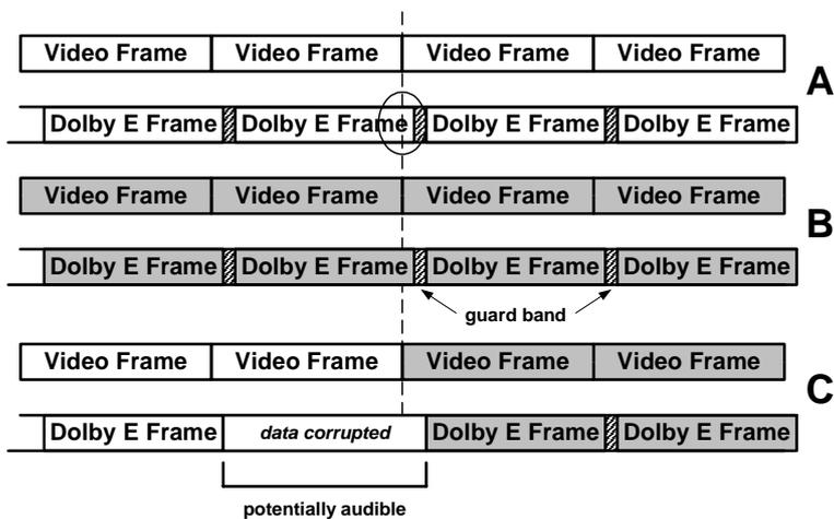
**Figure 5-6** Switch/Edit of Non-Phase-Aligned Dolby E Bitstreams (Example 1)
