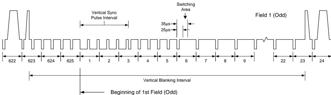
**Figure 4-2** PAL Composite Vertical Blanking Interval
