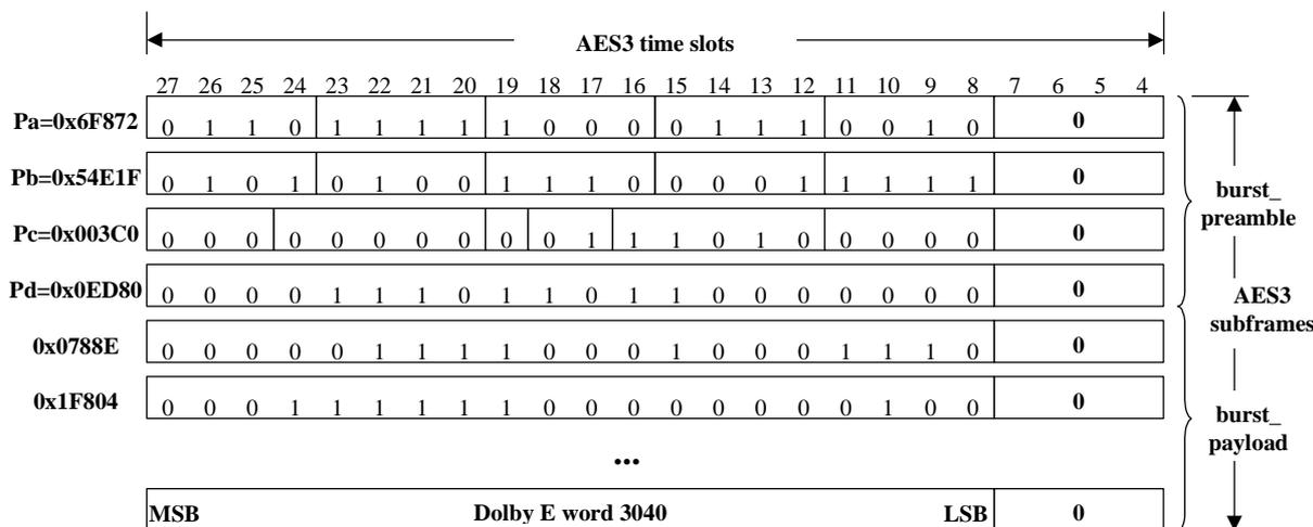
Figure 4-9 Example Mapping of KLV Data Burst to AES3 Time Slots
