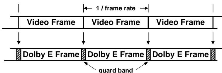
Figure 5-3 Phase-Aligned Dolby E Frames
