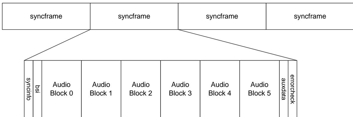
Figure 1: Section of a Dolby Digital bitstream
