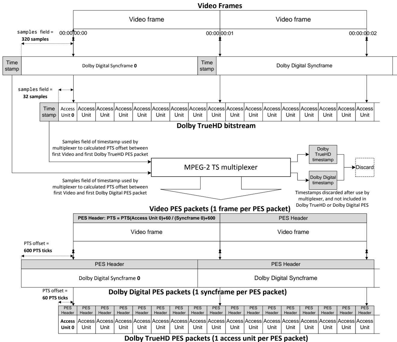
Figure 15: Use of SMPTE timestamps to specify initial A/V offset for BDMV MPEG-2 TS
