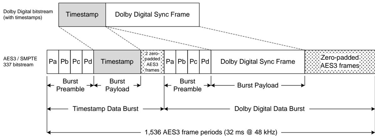
Figure 16: Formatting Dolby Digital bitstream with SMPTE timestamps for SMPTE 337 transmission
