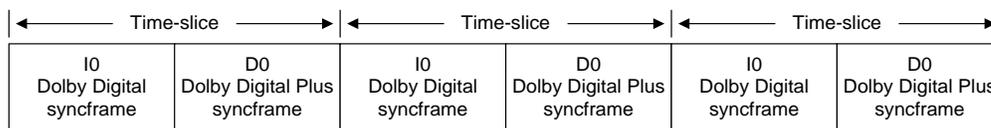
Figure 5: Dolby Digital Plus primary audio bitstream on a Blu-ray Disc with IO Dolby Digital syncframes and D0 Dolby Digital Plus syncframes
