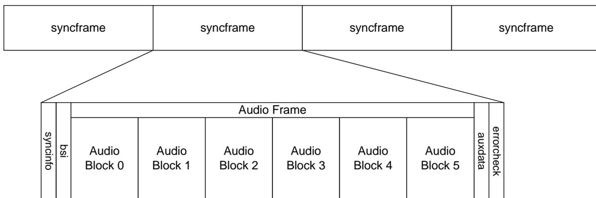
Figure 2: Section of a Dolby Digital Plus Bitstream (six audio blocks per syncframe shown)
