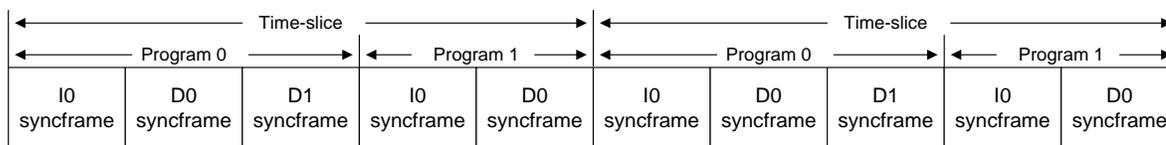
Figure 7: Dolby Digital Plus bitstream carrying two programs with IO, D0, D1, I1 and D0 syncframes
