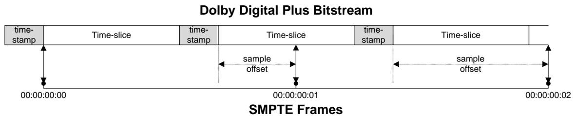
Figure 12: Timestamps and sample offset relationship in a Dolby Digital Plus bitstream
