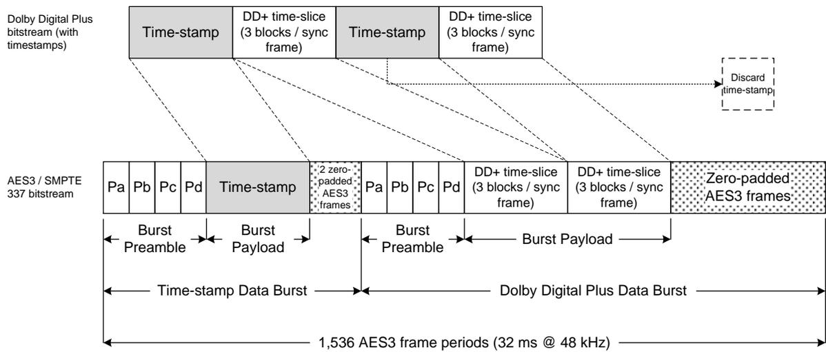
Figure 17: Formatting Dolby Digital Plus bitstream (3 blocks / syncframe) with SMPTE timestamps for SMPTE 337 transmission
