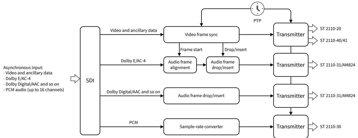
As with a traditional gateway, a video frame synchronizer is required to bridge the two clock domains. This involves the insertion of repeated video frames to maintain consistent latency. For encoded audio, including Dolby E or AC-4, a similar approach must be taken, where frames are inserted or dropped.
