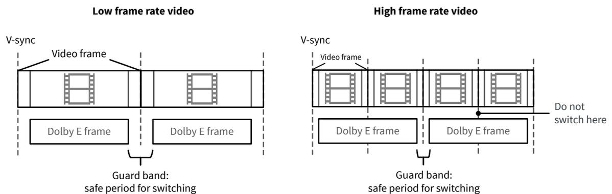
Figure 6: AC-4 safe switching point
