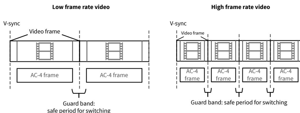
When a Dolby AC-4 stream is switched or frame drops and insertions occur, the Dolby AC-4 encoder must be in a mode where the Dolby AC-4 encoder creates independently decodable audio frames only.
