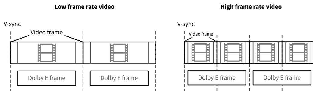
When distributing AC-4 (for example, in an SDI environment), and the AC-4 frame rate equals the video frame rate, audio frames must be phase locked to video frames as shown in this figure.
