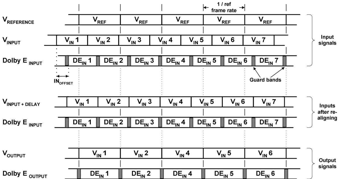
Figure 1: Example of frame synchronisation with Dolby E
