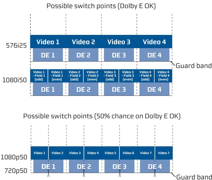
Figure 1. Interlaced Video and Dolby E (top), Progressive Video and Dolby E (bottom)
