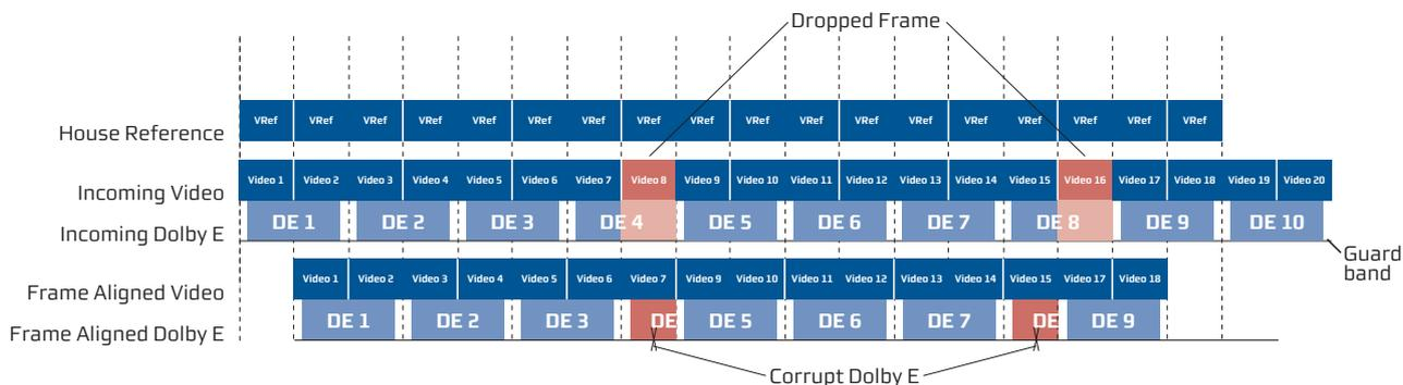
Figure 3. Progressive Frame Synchronizer Locking to Progressive Reference
