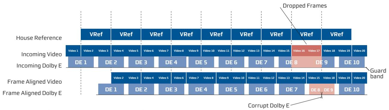
Figure 4. Progressive Frame Synchronizer Locking to Interlaced Reference
