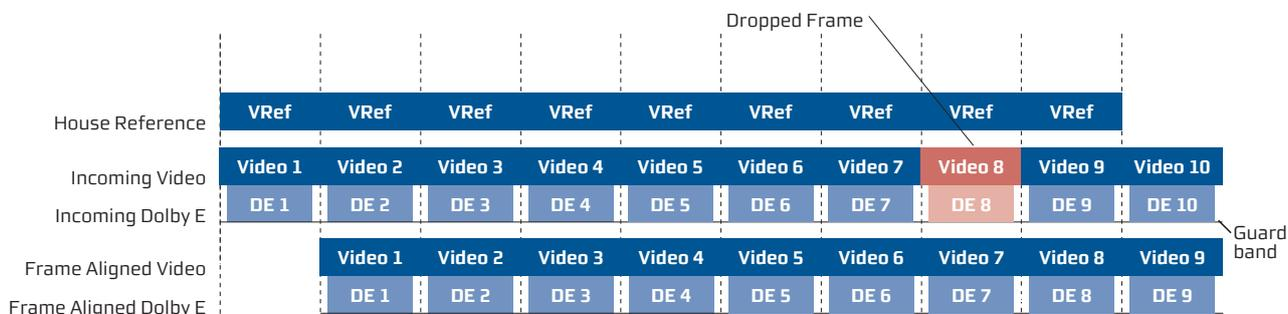
Figure 2. Standard Interlaced Frame Synchronizer Locking to Interlaced Reference
