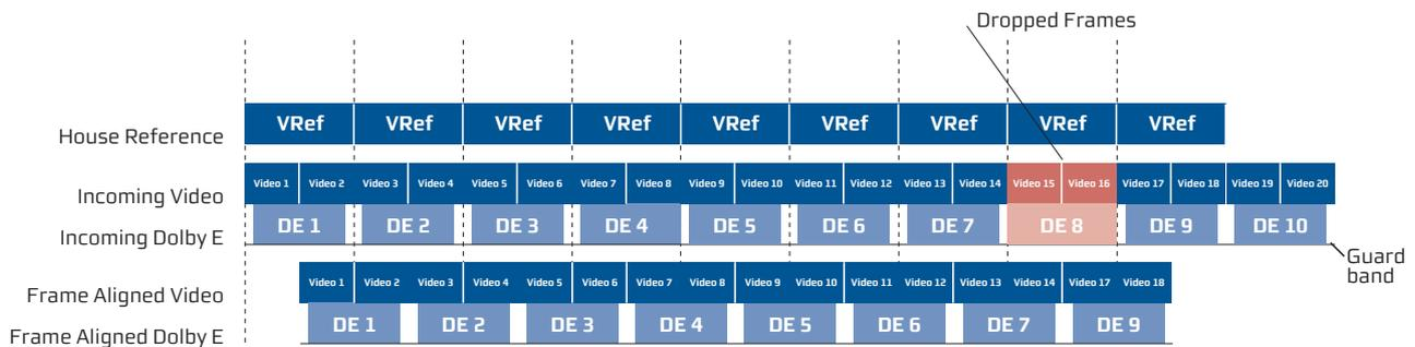
Figure 5. "Dolby E Safe" Progressive Frame Synchronizer Locking to Interlaced Reference
